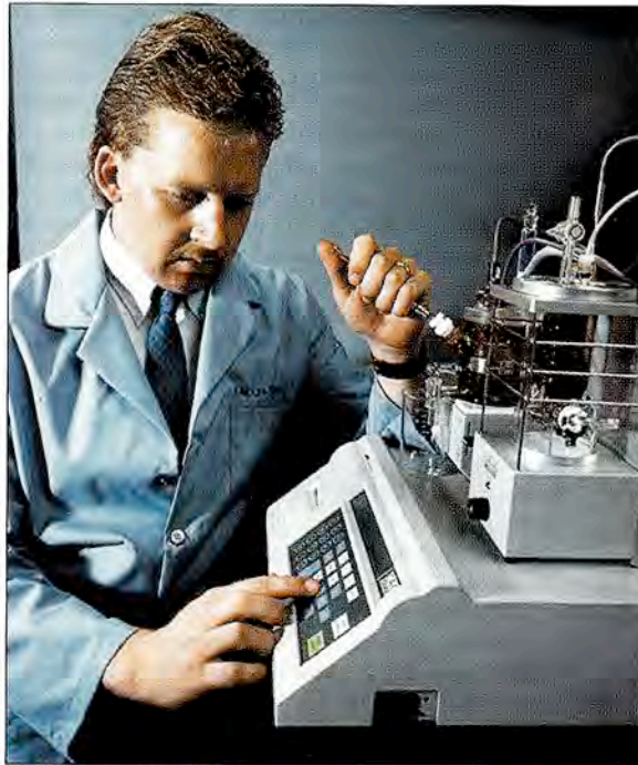
Oilpure lab technician Scott Severt uses moisture titration to quantify the amount of water in an oil sample. Water is the most damaging, yet least checked for, oil contaminant.
