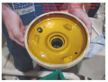
Electrostatic Charge on Filter Housing Metal Surface
