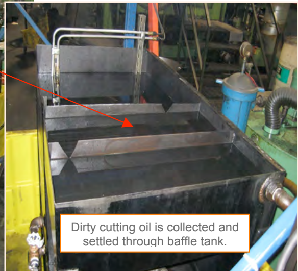
200 Gallons per week of Fuchs 346 cutting oil at @$8 per gallon, has been recycled by FC-4-SS-50 oil recycling machine. Zero cutting oil and compressor oil discharge from Gardner Denver plant with OilPure Systems.
