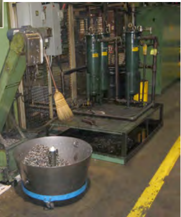
200 Gallons per week of Fuchs 346 cutting oil at @$8 per gallon, has been recycled by FC-4-SS-50 oil recycling machine. Zero cutting oil and compressor oil discharge from Gardner Denver plant with OilPure Systems.
