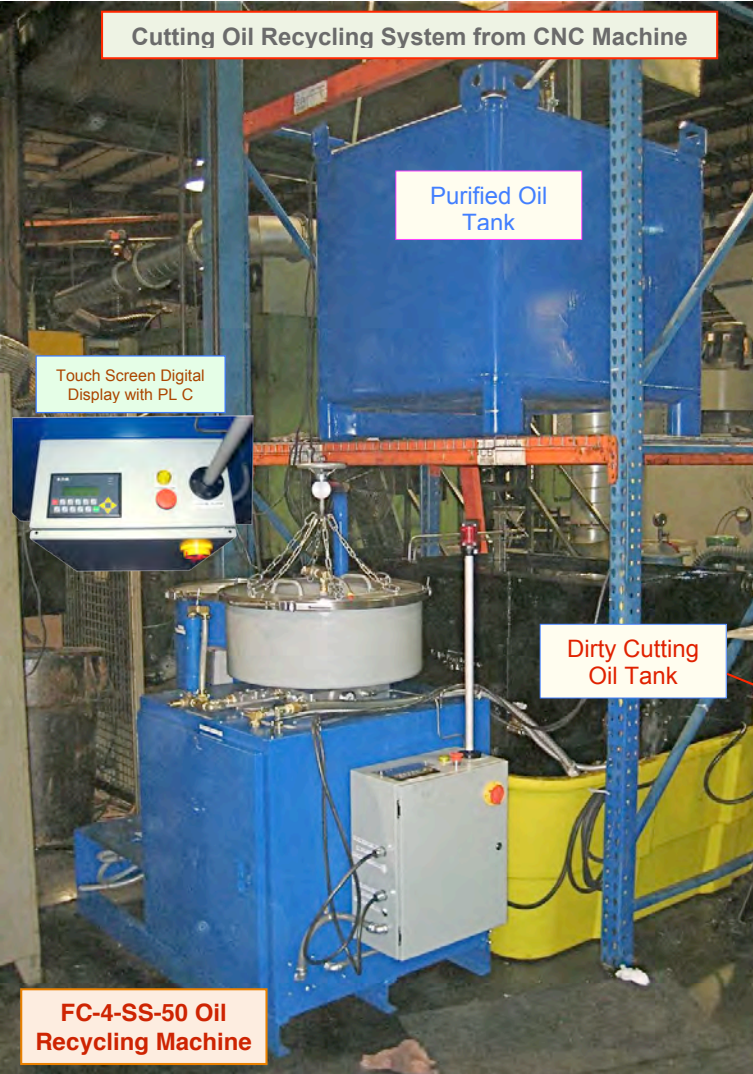
200 Gallons per week of Fuchs 346 cutting oil at @$8 per gallon, has been recycled by FC-4-SS-50 oil recycling machine. Zero cutting oil and compressor oil discharge from Gardner Denver plant with OilPure Systems.
