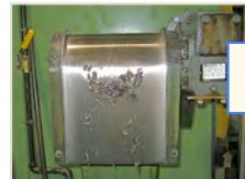
100 Gallons per week of compressor oil, at @$10 per gallon, has been recycled through MB-50 oil purifier.
